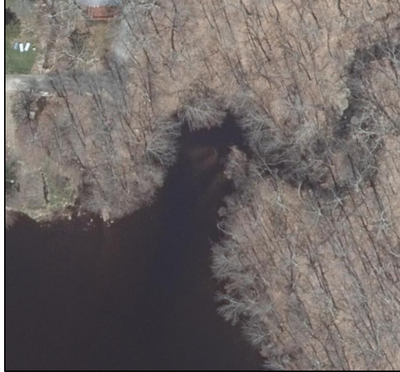
Figure 3: 2019 CT Aerial Photography showing sediment deposition at the main tributary inlet.
